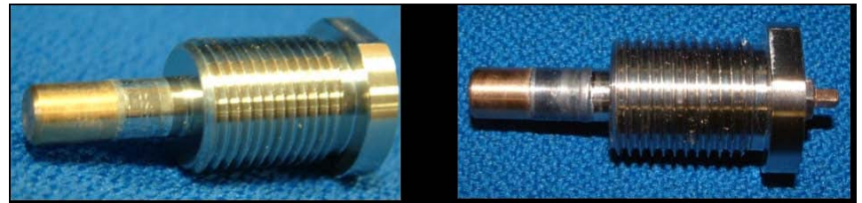
Aluminium/copper seal combination (left); Lead/copper seal combination (right).
