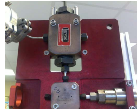
Harwood C-4133 H2 10Kbar valve assembly on Centre-Stick
